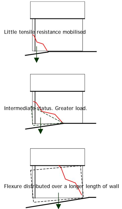
Cantilevers and building failure. Top we have relatively little weight overhanging a short distance. The bending moment is less than the case below it.
