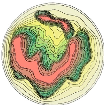
PRD Root Zone on Plan with variable soil stress related to moisture content.
